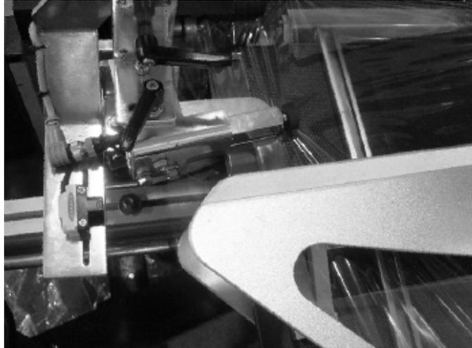
The rubber-covered tension rollers above and below the infeed conveyor have the task of feeding the film, free of folds, through the end-sealing unit and into the Length-sealing unit. The axles of the tension rollers should not be exactly perpendicular to the direction of film movement; viewed from above, they should be rotated counter-clockwise by a few degrees. The optimum adjustment depends upon the type, width and thickness of the film and must be determined by experiment in test runs.
