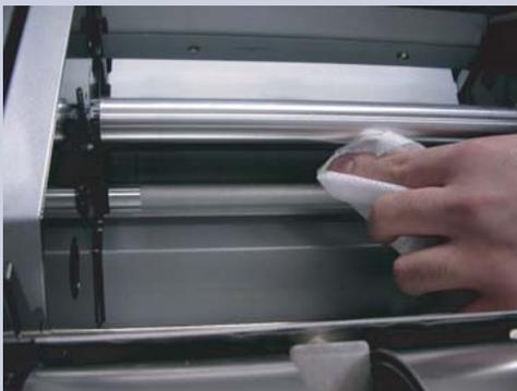
You will be able to see the folding roller when you release the bottom lever of the folding unit.
