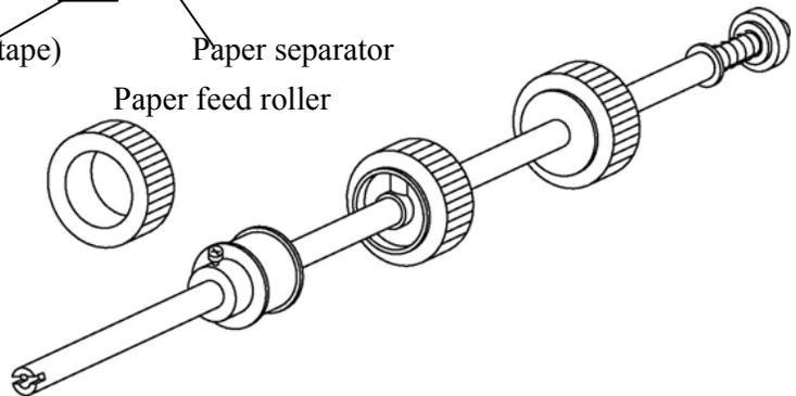
Grasp the paper separator (with plastic part) at both ends and pull it out. To install, reverse the procedure.
