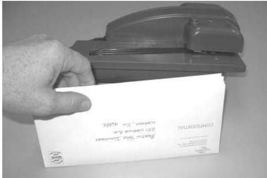
**Step 1.** Prepare up to 10 standard envelopes to be opened by tapping the top sealed flap side down firmly on desktop several times. This will cause the envelope contents to slide to the opposite side of that to be opened.
