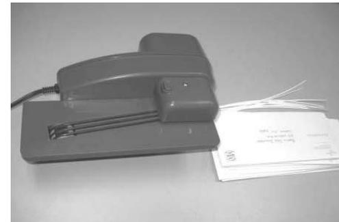
**Step 5.** Your stack of envelopes will be stacked on the right side of the unit and the scrap is easily separated from your opened envelopes. The cut edges of your envelopes are cut such that they are unlikely to cut or injure fingers.
