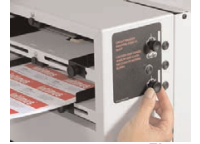
Fig. 7 Adjusting the retarder
