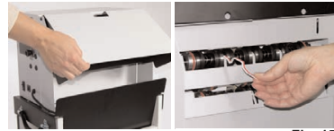
Fig. 14 Lifting the rear assembly
