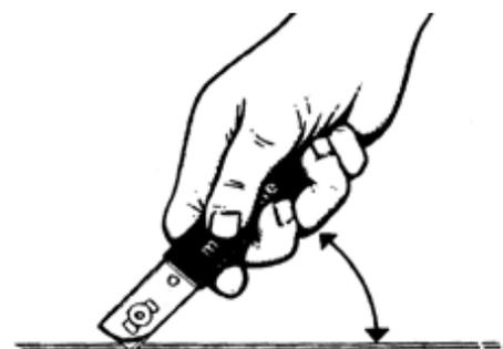
If you are cutting across a sheet of matboard, simply start the blade beyond the top edge of the board and pull the Mat Knife completely through.
