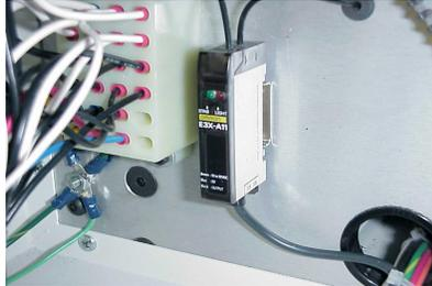
1. Remove front cover from the photoelectric switch.
