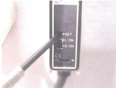
8. The Sensor should be adjusted properly.
