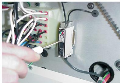
5. Turn the adjusting screw counter clockwise until you hear small clicking sounds and the little green light is the only light on.
