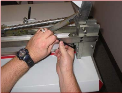
Photo 1-Blade handle must be properly positioned to get access to the outer Allen screws.
