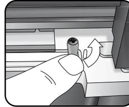
Rotate small safety catches to release the cutting strip. Turn cutting strip over to use other side of the strip. When all areas have been used, replace cutting strip with new one from accessory pack (#54125). Re-secure cutting strip and **SafeCut™ Guard** again.
