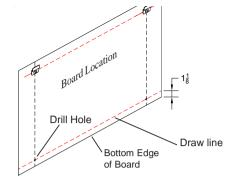
Lift and remove board from the Z-Hangers. Measure up from bottom line of board 1-1/8", and draw line as shown. Locate stud near each end of board and drill pilot hole along line using 1/8" drill bit.
