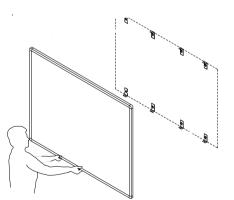
5 Secure top Angle Brackets (A) to the wall using long screws (B) as shown. Follow diagram in Step 1. Set board on the bottom angle brackets.
