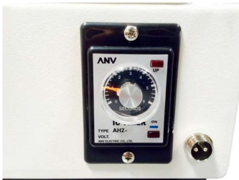
Figure 12. Remove the old timer
