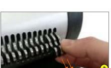
3. Disengage pins that would punch off the edge of the document by pulling them towards you. TIP: Punch a few test sheets first in order to get the proper alignment.
