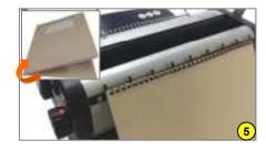
5. Position the wire on the wire holder. TIP: Flip the back cover over to make it face the front (see inset) then insert into the wire making sure all teeth go through the holes.
