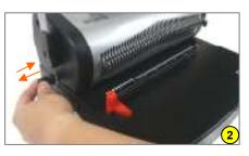
2. Adjust depth margin control from 2.5mm to 6.5mm. This controls how far or how close you want the holes to be in relation to the edge of the document.
