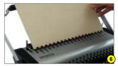
6. Insert the document into the comb making sure all teeth go through the holes then release the handle to close the comb.
