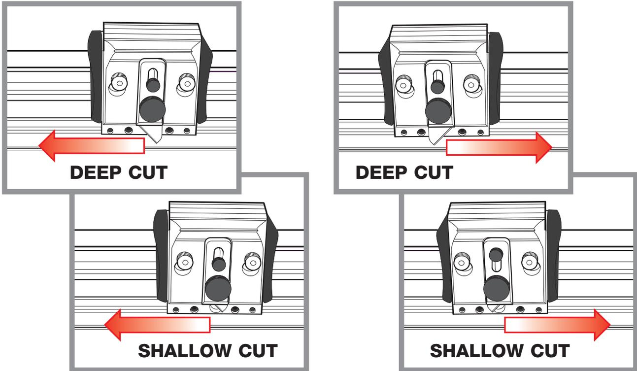
Once the blade is set move the cutting head near to the start of the cut, press down the blade holder and push or pull to make the cut. Only light finger pressure is usually required to depress the blade holder so most of your effort can be directed into pushing the blade through the material.
