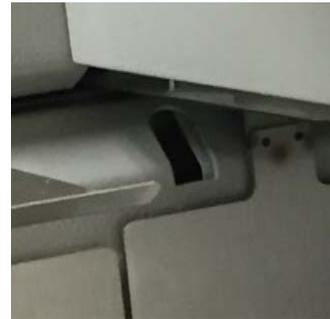
**2. front guide knob-** Turn the knob clockwise to decrease the gap (shown in illustration below) if double feeding occurs, or turn the knob counter-clockwise to increase the gap if the paper is unable to pass through.
