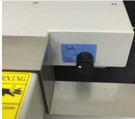
**Skew adjustment-** Using the knob shown below the user can adjust for any skew in the crease or perf of the sheet. If the wheel is turned downward the feed table will move to the left. If the wheel is moved upwards the feed table will move back right. Generally if the paper is perfectly square no adjustments need to be made.
