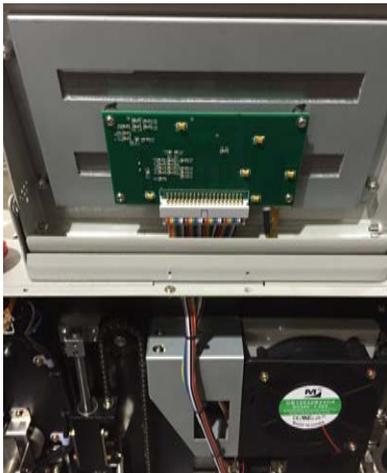
Next, Remove the back cover from the touchscreen. It will take four screws that are located on both sides.
