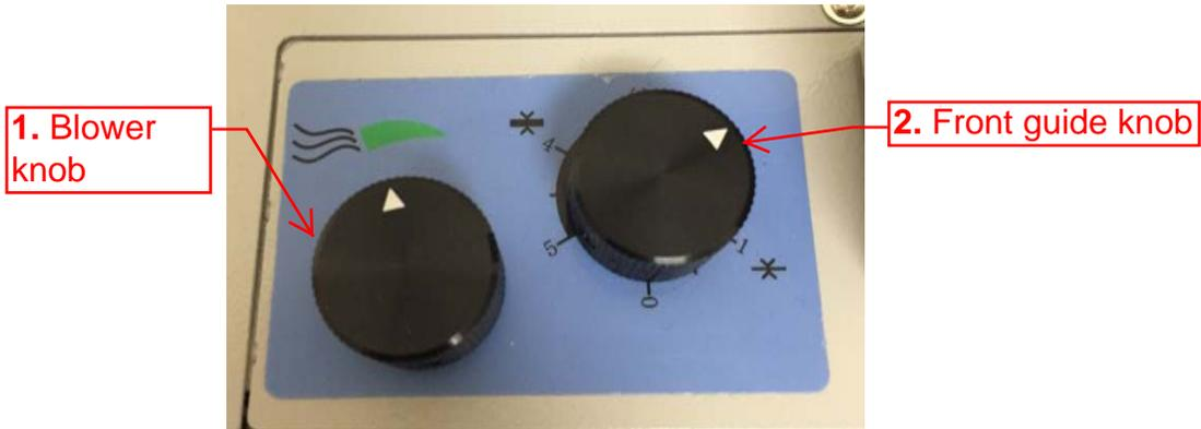
**1. blower knob-** Turn the knob clockwise to make the air vents smaller (see image underneath to left), and counter-clockwise to increase the air vent sizes (see image underneath to right). If stock is thin, the air vent size should be smaller, air vent sizes should increase as paper thickness increases. This air adjustment is important for proper feeding. If a sheet is not being picked up by the belt to feed please adjust the air.
