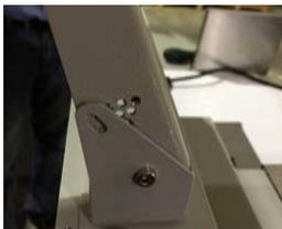
Change the angle of the touchscreen by putting the side screws in the appropriate location for ease of use.
