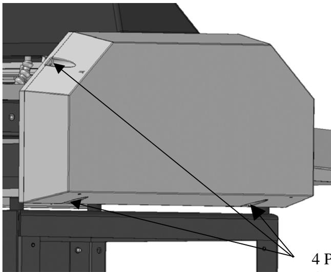
Begin procedure by removing the Non-op side cover.
