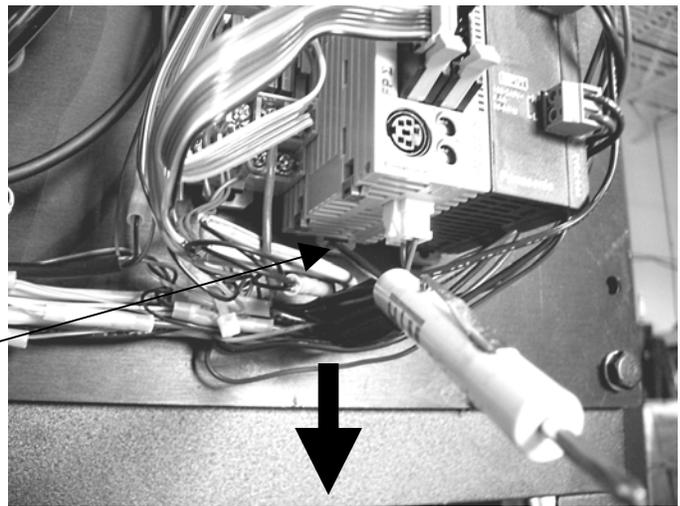
The battery is located under a cover located at the top rear of the Plc controller. Insert a screwdriver into slot and pry cover off unit
