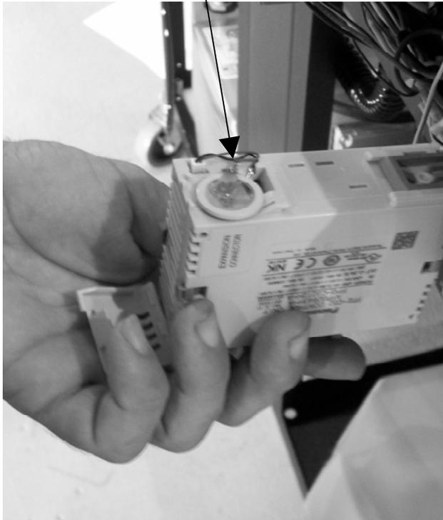
**With the POWER ON**, unplug the old battery and remove. Replace with new battery. Install the battery cover and place unit back on din rail. Be sure to push locking tab up to lock unit in place. Replace Non-op side cover and unit is ready to continue operation for another 2 years.
