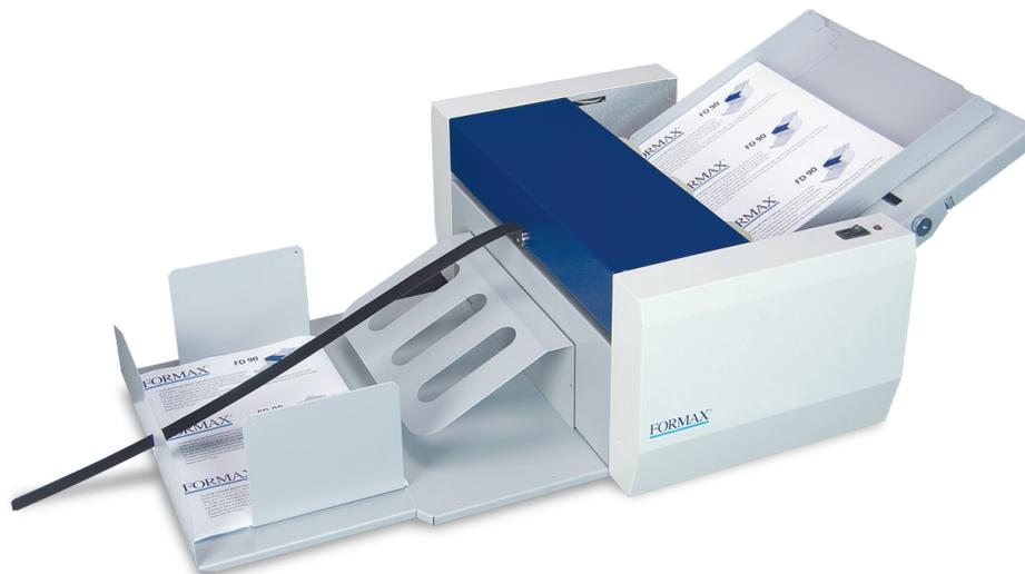
The **FD 90 Rotary Perforator/Creater** is specially designed for finishing printed sheets, up to 13.8" x 19". Its three-tire friction feeding system reliably feeds up to 6,800 sheets per hour, and can create up to 5 parallel perforations and/or creases in a single pass. Perforating allows for easy separation of multiple printouts, tear-offs, postcards or tickets on a single sheet, while creasing allows for easy folding and reduces unsightly cracking in digital printouts.
