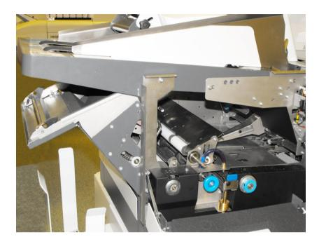
If paper is not fully visible, turn blue knobs to wind into view.
