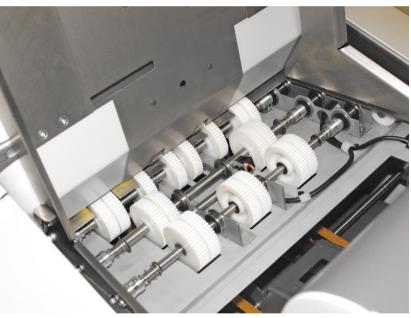
Slide spring-loaded collars inboard and lift feed shafts out of their bearing hubs. The feed tyres can be prised off the rollers and replaced with alternative items.
