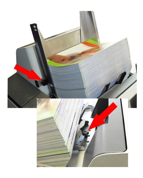
Slacken side-guide knob and adjust guides to 1-1.5mm clearance each side. Tighten knob.
