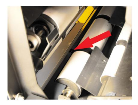
Open side cover and lower front output cover below envelope feeder.
