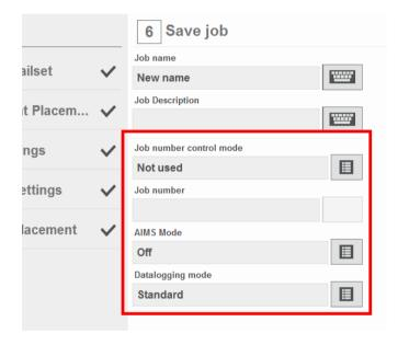
24 Set the **Job number control mode.** Options are Auto generated; Manual entry (Internal or External); Read from prime; Read on output; Externally supplied.
