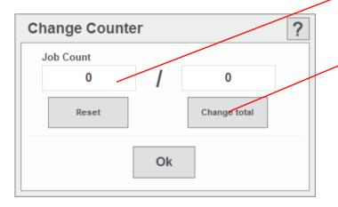
Current job until changed, even if switch-off/back on. Press **Reset** to zero.
