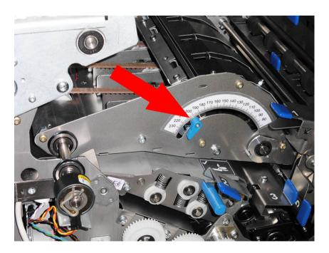
Open side cover. Slacken knob and set to length on scale.
