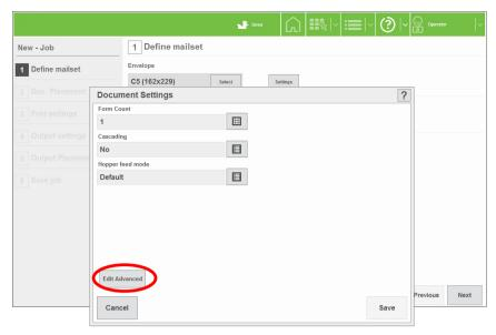
10 Set form count for multiples, and if required, select cascading (automatically feed from another hopper when this one runs out), or Daily Mail (hand-feed) or External feed (FFPD).
