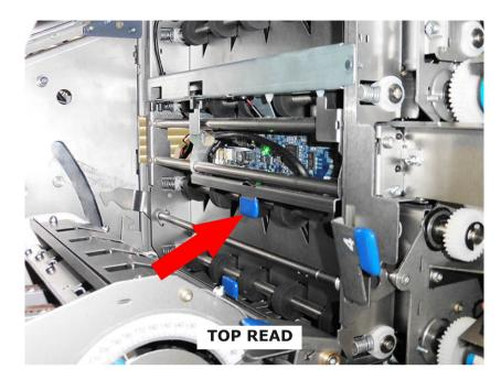
Open side cover and using blue tab, slide CIS reader over to the side of the paper that the label is printed.
