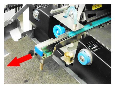
Open the side cover on the insert head. Using the blue tab, lift the end of the wetter tank slightly and withdraw it.
