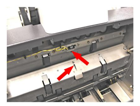
Open perspex top cover and raise collate clamshell (closest to envelope hopper) so it locks in place.
