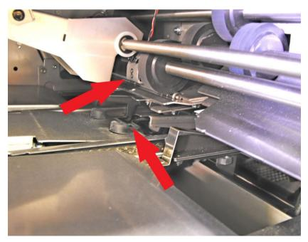
Lower side cover and raise overguide inside closer cavity, latching it in place.
