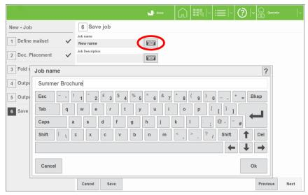
Press the keyboard button and enter a job name using virtual or physical keyboard.
