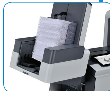
High-Capacity Vertical Stacker holds up to 500 filled envelopes
