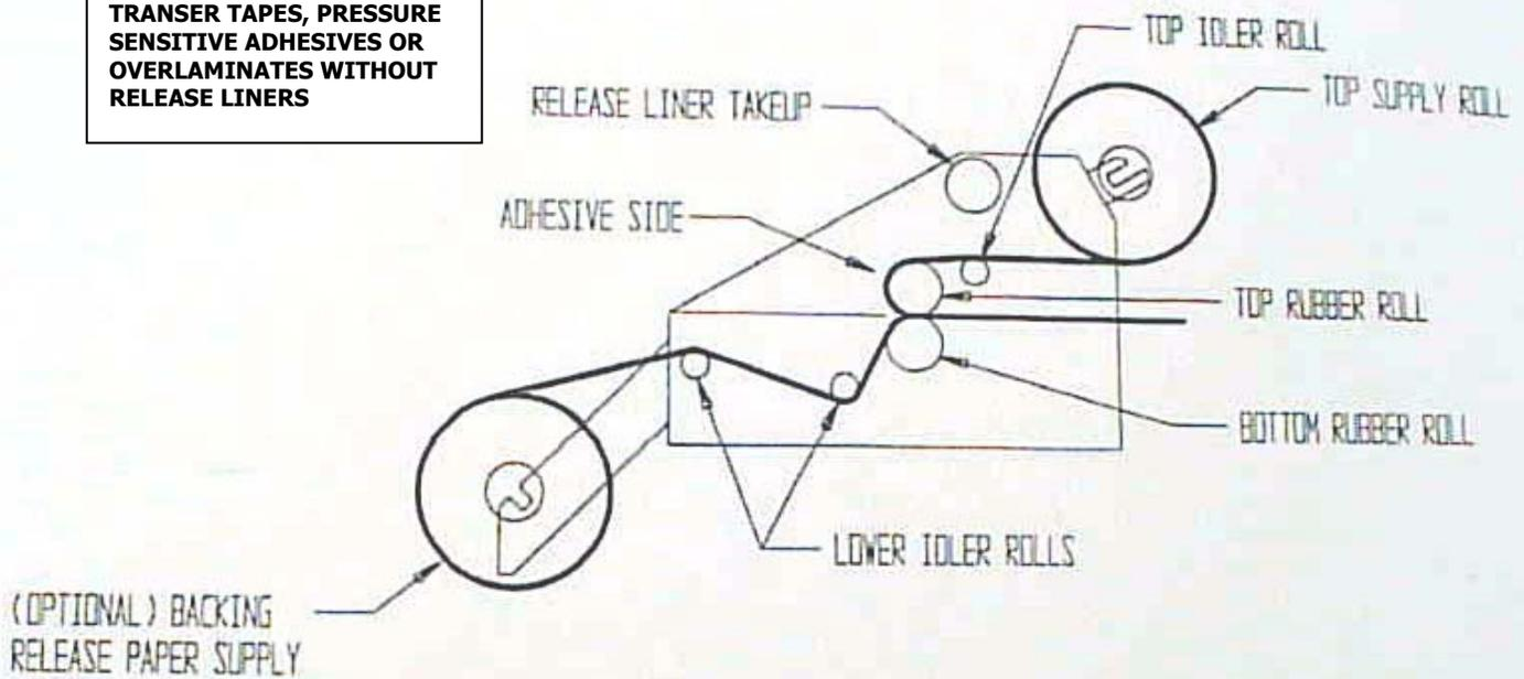
NOTE: The operator must use a backing paper either from a supply roll or in sheets to prevent adhesive from adhering to the machine
