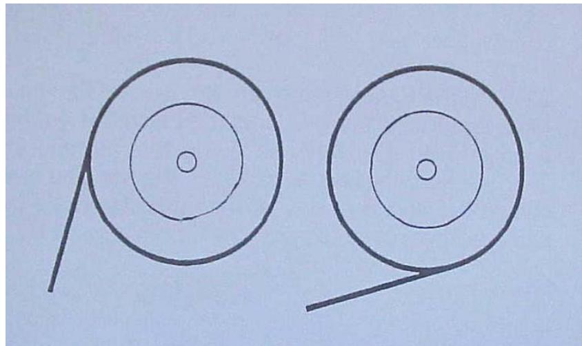
2. Center the roll on the mandrel and place the mandrel in the top brackets. This is a job best done with two people, even if the roll of film is not very heavy. With a person holding each end of the mandrel, it is easy to put both notch fittings into their respective brackets. Make sure they are both fully seated. Attempting to load the PSA material on the laminator by yourself may result in a back strain or other injury.
