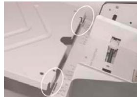
To install the Extension onto the Exit Conveyor, align the tabs on the Extension with the slots provided in the Exit Conveyor as shown. No force is required to install the Extension - gravity will hold the Extension in place.
