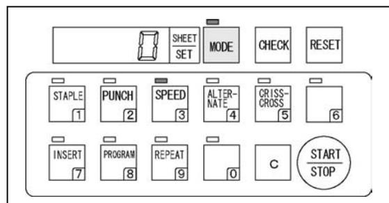
(2) Press the **SPEED/3** key to change speed. Each time the **MODE** key and **SPEED** key are pressed, speed switches between high and low speed.
