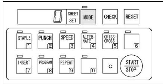
(2) Press the **ALTERNATE/4** key for Alternate mode. Each time the **MODE** and **ALTERNATE/4** keys are pressed, the mode switches between them.
