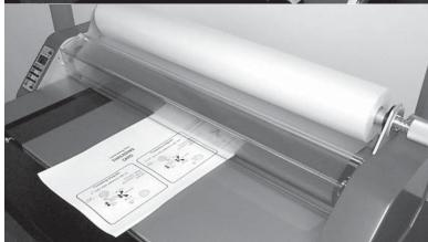
Slide the top and bottom film rolls from side to side on the mandrels so that the film is perfectly aligned top and bottom (Note: overlap will cause the film to deposit residue on the heat shoes and rollers, so this procedure is critical). Replace feed tray and heat guard.
