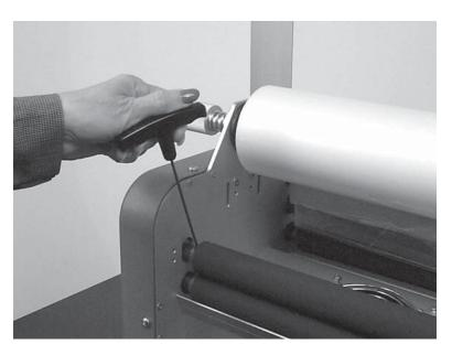
**Shut the machine off!** SL27's have set screws at both ends of each laminating and pull roller. With the use of a 3/32 hex key, loosen all four set screws on the pull rollers. Cut the plastic between the laminating and pull rollers, grab the loose end and pull. The rollers will rotate freely on the roll shafts and the "wrap-around" will easily unwrap. Tighten all the set screws and rethread the film.
