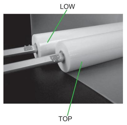
Load the mandrel on the laminator by inserting the slot end of the mandrel into the tension adjuster on the right side and then lowering the hanger end into the bracket on the left side.
