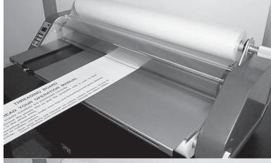
Start the motor by pressing the "Fwd" button. Feed the threading board and film in between the heat shoes. This will pull the film through the rollers until it comes out the back of the laminator.
